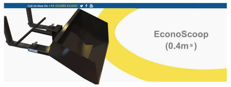
To fill the bucket and pick up a load of material, the material should be approached with the bucket at ground level. The truck is driven carefully forward, with the mast as near upright as possible until the bucket fills. The forks can then be raised and the material transported as required. To dump the material, the bucket is positioned directly over the discharge point. Once correctly positioned the operator lifts the release lever and the contents are discharged.
